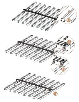
6. Insert the M6 screw and nut into the support frame at first, but do not tighten your screws (Fig.i); Leave space between the nut and support frame. Slide them into the light track (Fig.j); Adjust the support frame to keep the balance, and then tighten the M6 screws.
